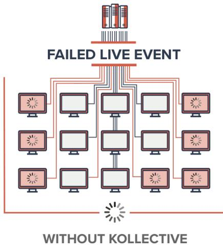
Many user's connecting simultaneously to live events saturate enterprise networks resulting in poor user experience.
